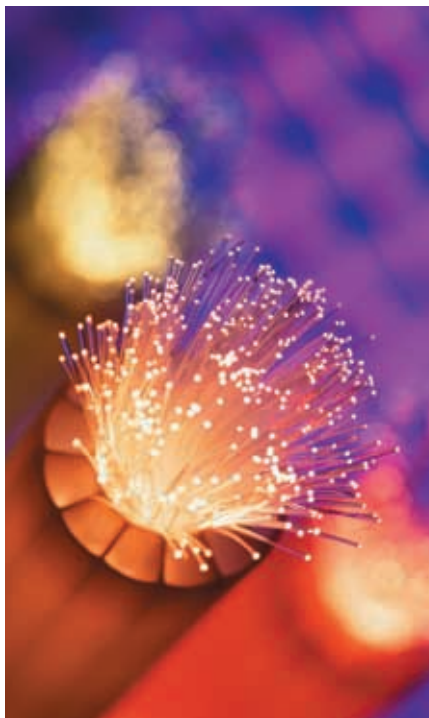
Fibre optic cables transmit signals faster over greater distances than copper wires. Each optic cable contains 96 fibre strands.
