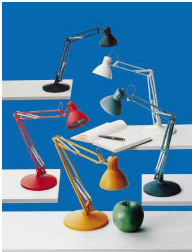
Lillyna is a variant of the L-1 Luxo luminaire, the world-famous precursor of all articulated self-balancing luminaires. The luminaire is supplied with an L-arm with external springs and a parallel motion feature, which always keeps the head horizontal to the surface. Over the years following its first appearance in 1937, the L-1 has notched up all the most prestigious prizes for industrial design.
